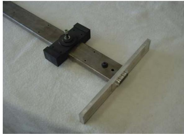
1 x 3 Tube Frame, Standard Body Bolster and End Sill
