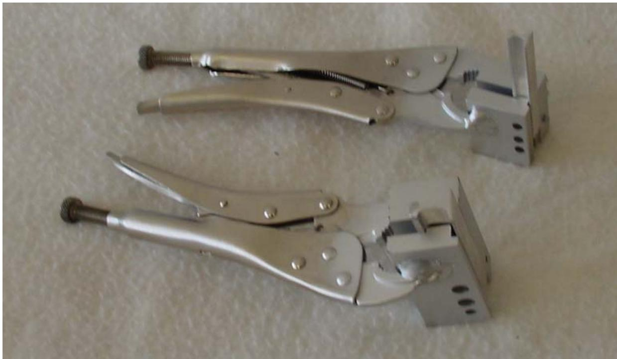
**Rail Drilling Jig** - Furnished Attached to the Jaws of Locking Style Pliers to Allow Secure Clamping to Rail. Design Provides a Flat Back for Use on a Drill Press Table and an Open Bottom to Allow Field Use on Rail Already Secured to Ties.
