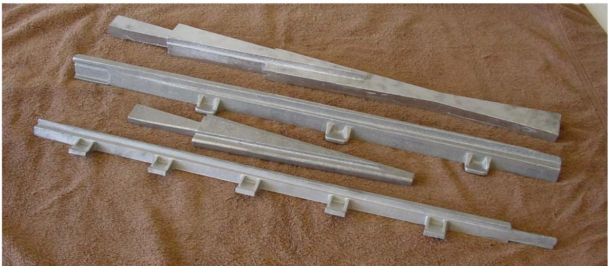
Cast Aluminum Point Pairs and Frogs for Switch Construction.
