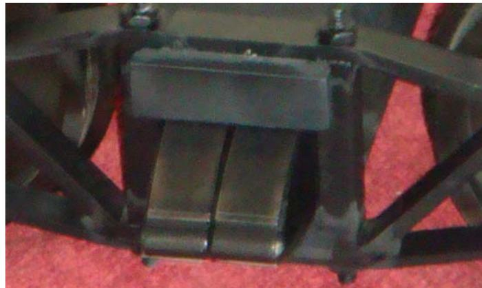
These are leaf spring conversion units for some of our trucks. Leaf springs were commonly used under cabooses, tenders, and other cars which carried people. Drawing shows conversion unit for Modern Roller Bearing and Steam Era Trucks. Photo shows leaf springs in Arch Bar Truck.
