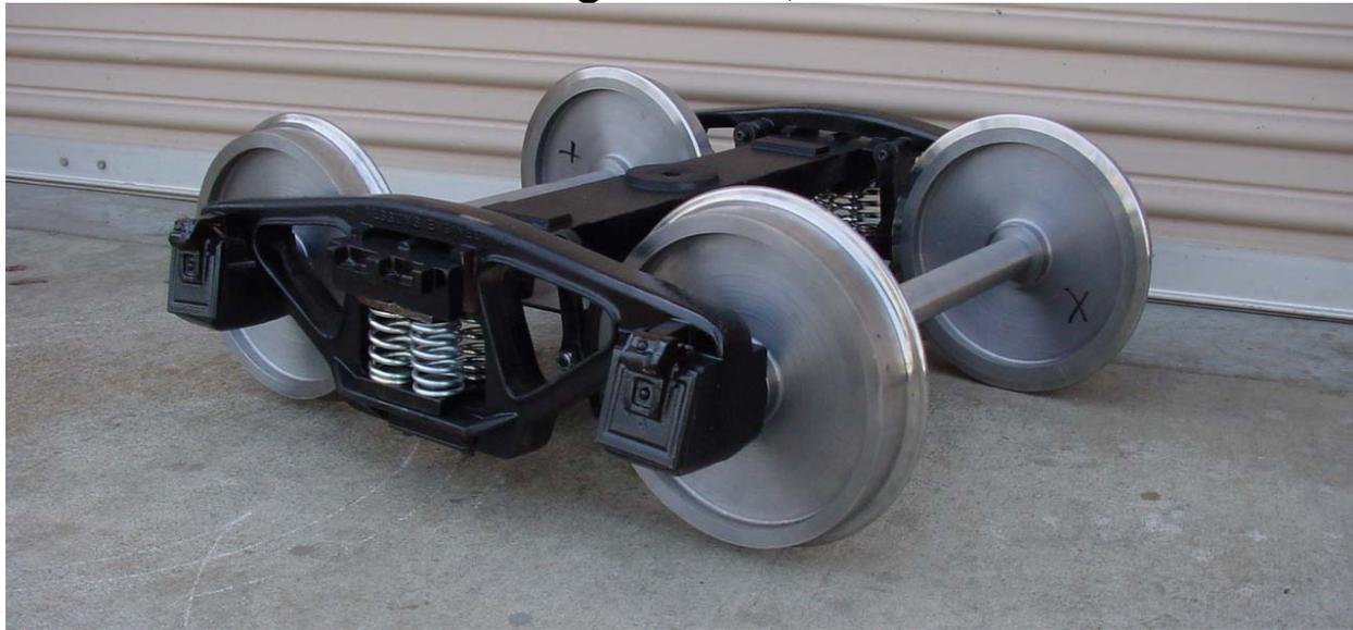
This truck was one of the most commonly seen designs from 1920 to the 1970's. Unlike most of our trucks, this truck is offered as a set of castings to make two trucks but does not include bearings, springs, or metal stock.
