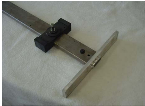
1 x 3 Tube Frame, Standard Body Bolster and End Sill Shown Upside Down
