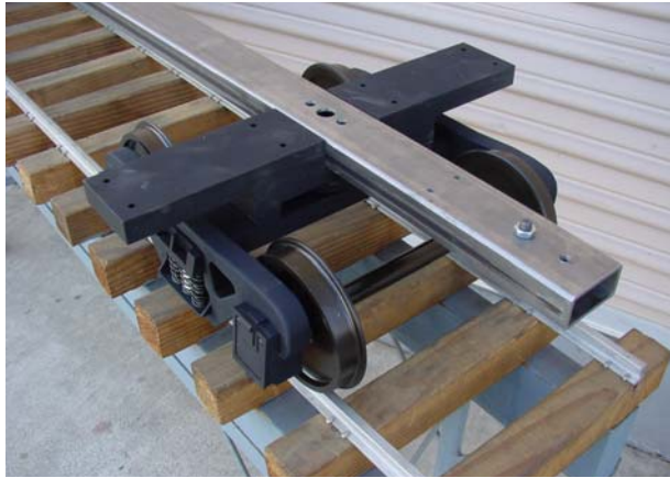
1 x 2 Tube Frame with Wide Body Bolster Shown Mounted to Trucks
